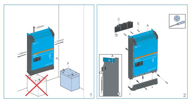
Refer to the Dimensions [32] chapter for the location and dimensions of the mounting holes.
